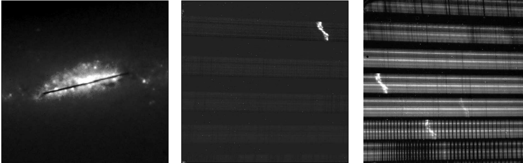
Figure 3. The official “first light” NIRSPEC target - M82. The left hand image is a 20s exposure in the KL filter with the slit-viewing camera. The central and right images show respectively, an L-band and a K-band echellogram. The slit is 24" long.
