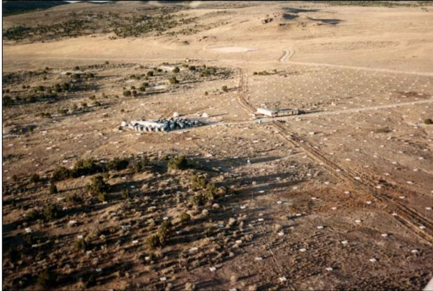
Figure 4: Aerial view of CASA-MIA showing the 1089 CASA detectors, surrounding the Flye's Eye II apparatus and two house trailers used for the CASA living quarters and laboratory (photo by Kenneth Gibbs).
