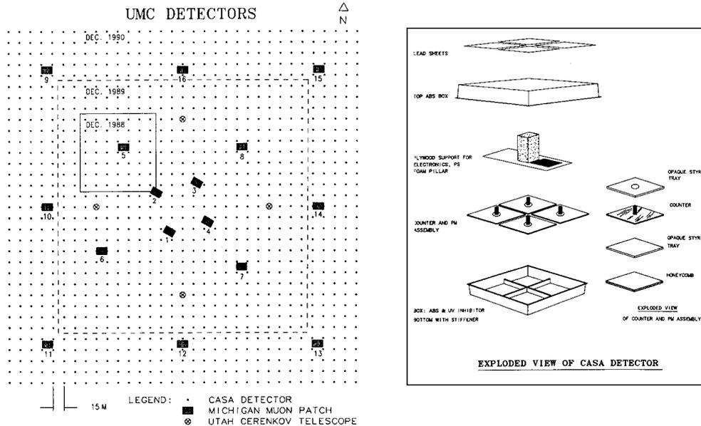
Figure 2: Left: plan view of the CASA-MIA experiment at Dugway UT, USA, consisting of 1089 surface detectors (CASA), 1024 buried muon counters distributed into 16 patches (MIA), and four small Cherenkov telescopes. Right: exploded view of a CASA station, consisting of four scintillation counters enclosed in a water-tight box and covered by four sheets of lead.
