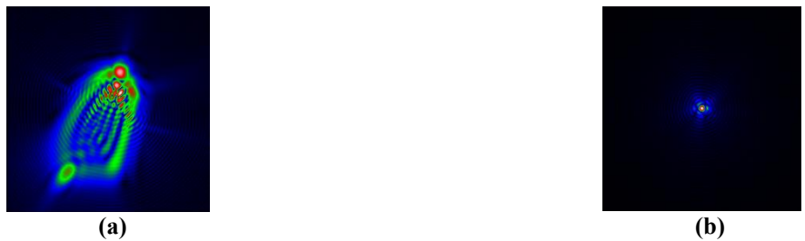
Figure 5: Focal spots of 633nm monochromatic light after transmitting through the aberrated optical system; (a) before; and (b) after the active optics compensation.
