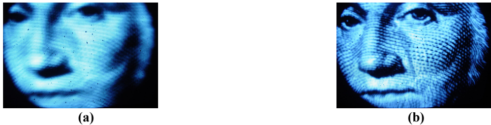
Figure 4. (a) An aberrated image (6.5 waves peak-to-valley at 633nm), and (b) compensation of aberrations with a 19-element deformable mirror (0.26 waves).
