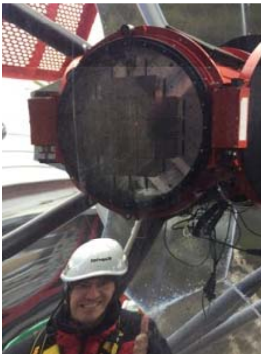
SST-2M-GCT Si-PM camera 75% complete (similar readout to SCT)
