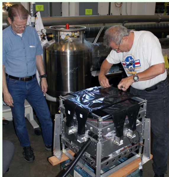
Installing TOF layer
