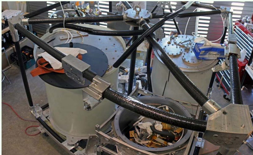
Detector, Si(Li) electronics, and pressure vessels
