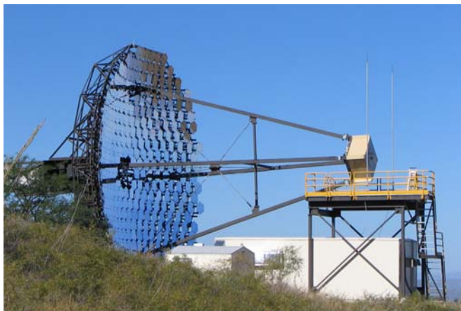
Figure 4: VERITAS Telescope 3 at the basecamp of Mt. Hopkins, Az, as of August 2006. VERITAS in an array of four 12m diameter imaging atmospheric Cherenkov telescopes starting scientific operation in January 2007.
